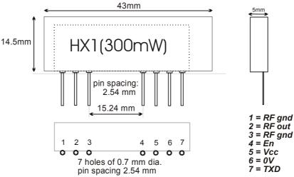
Figure 3: HX1 pin-out and dimension
