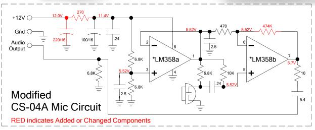
After replacing the 56K feedback resistor on LM358b with a 474K resistor the
